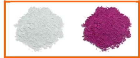
The **colorants** come in two main classes – dyes, which are soluble in the liquid carrier, and pigments, which are solid particles dispersed in the liquid carrier. From the environmental impact point of view, dyes are produced via a chemical manufacturing process, while pigments require large amounts of energy to grind the original materials to the correct particle size.
